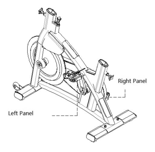
**Step 3:** Install the front and rear adjustment tubes, turn the knob counterclockwise and pull the knob outwards, and insert the front and rear adjustment tubes into the large frame at the same time, turn the knob clockwise to tighten.
