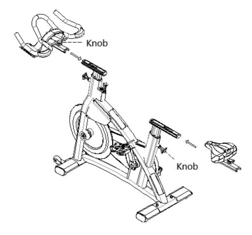
**Step 5:** After the installation is complete, the 4 feet are leveled. The reluctance knob rotates clockwise to increase resistance, and counterclockwise to decrease resistance. According to your height, adjust the height of the front and rear adjustment tubes, and adjust the distance between the handlebar and the seat according to your height.
