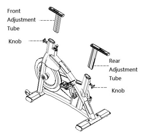
**Step 4:** Install the handlebar and seat. Push the handlebar and seat forward and backward according to the arrow direction. Turn the knob clockwise to tighten and counterclockwise to loosen. Adjust distance between the handlebar and seat according to your height.
